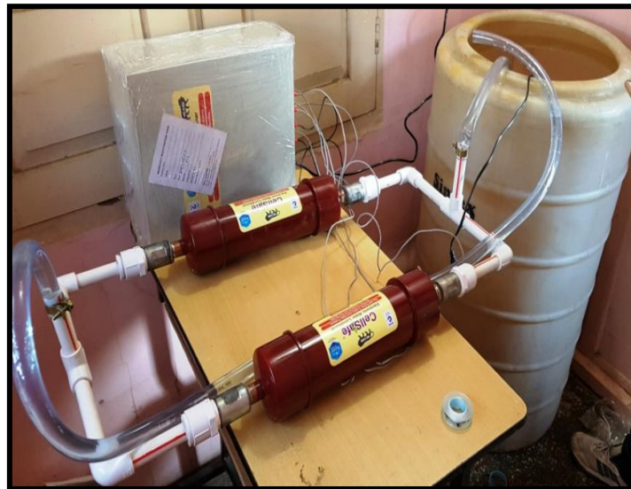
Fig 1. Setup of magnetic water conditioner
