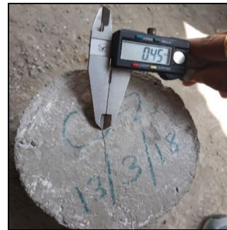
Fig 4.4 Checking of crack closing width using Vernier Caliper
