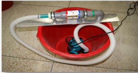
Fig. 7. Immerse-able pump used to circulate water through the magnetic field (Magnetizer).
