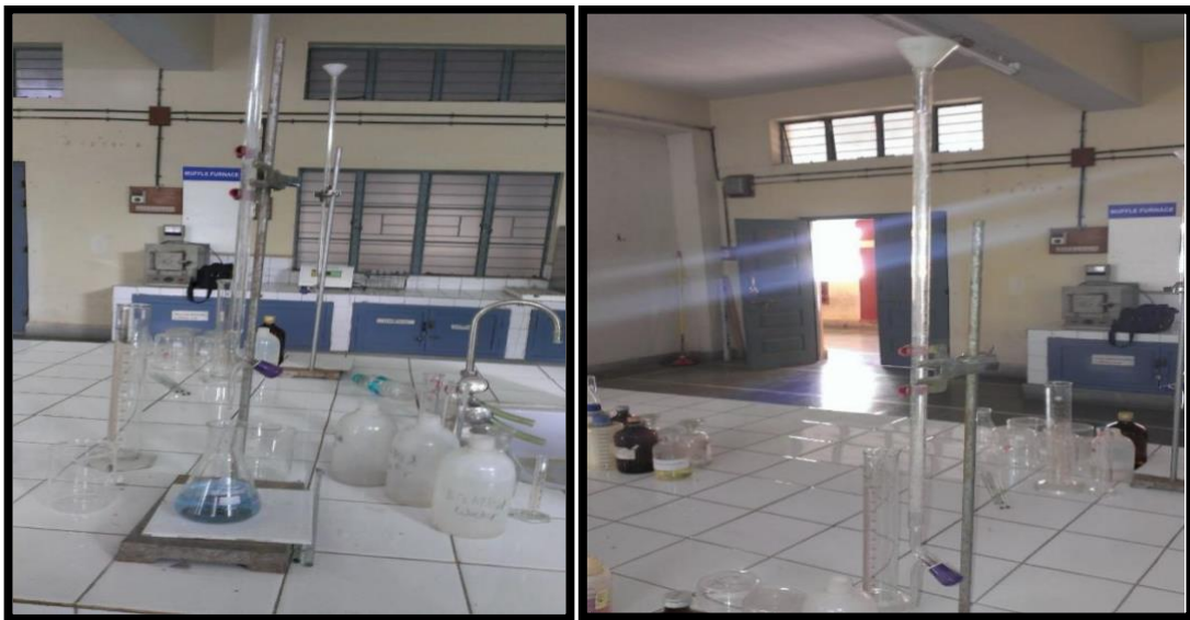
FIG 5.2 DETERMINATION OF HARDNESS OF WATER (TITRATION WITH EDTA) (A) ONGOING TITRATION (B) TITRATION APPARATUS
