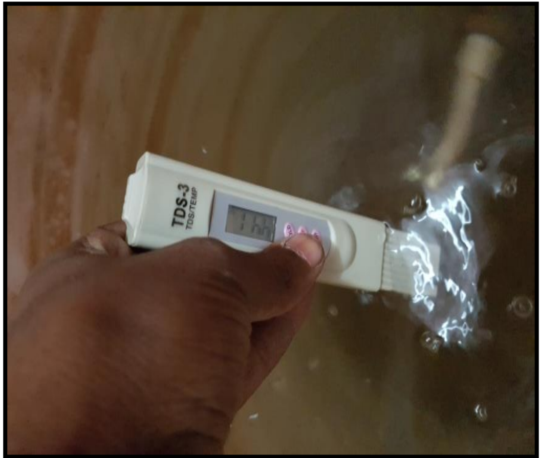
FIGURE 5.1 HM DIGITAL PORTABLE HANDHELD TDS METER SHOWING READING OF 441 PPM
