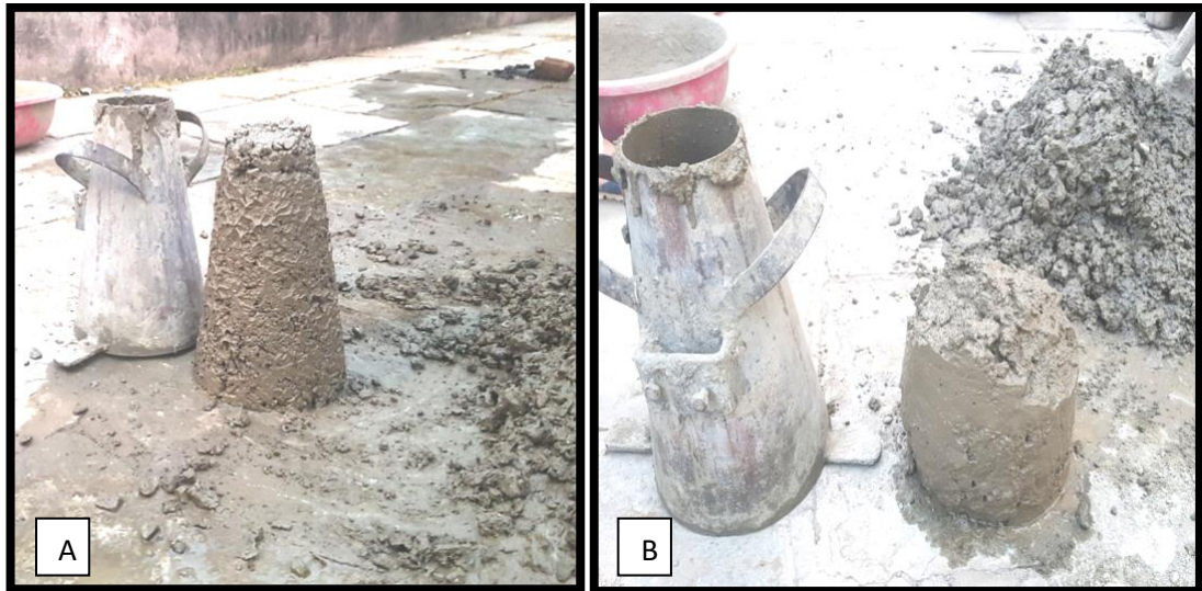
FIG NO 5.7 A) NORMAL WATER SLUMP
