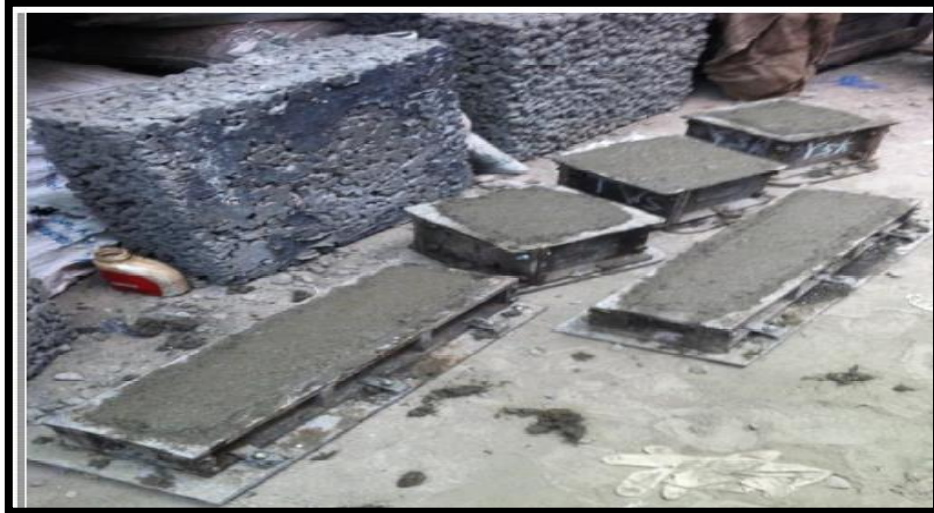
FIGURE NO 5.8 CASTING OF BEAM AND CUBE MOULDS
